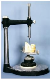
Fig. 5.5 Diagram of a cast surveyor. A, base; B, vertical rod; C, horizontal beam; D, vertical spindle; E, clawl for surveying teeth; F, a leveling rod; G, cast-rod; H, table of surveyor.
