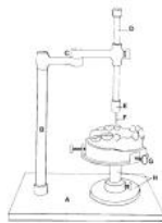
Fig. 5.5 Diagram of a cast surveyor. A, base; B, vertical rod; C, horizontal beam; D, vertical spindle; E, clawl for surveying teeth; F, a leveling rod; G, cast-rod; H, table of surveyor.
